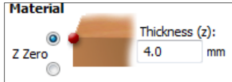
Figure 54: Vectric Z Zero Position
