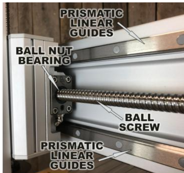
Figure 6: Weekly (best case daily) cleaning and application of light oil externally to screws and rails with cloth and light oil.
