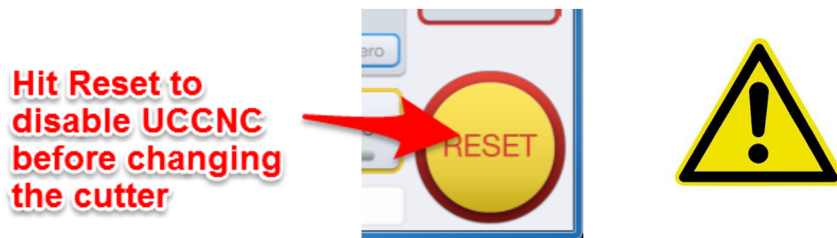
Figure 50: Reset to disable spindle relay
