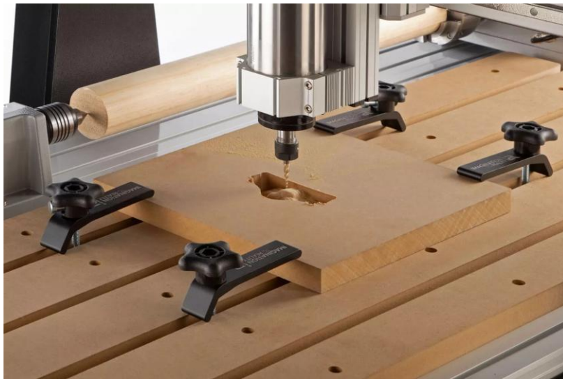
Figure 1: Clamping methods – Sheet Clamping
