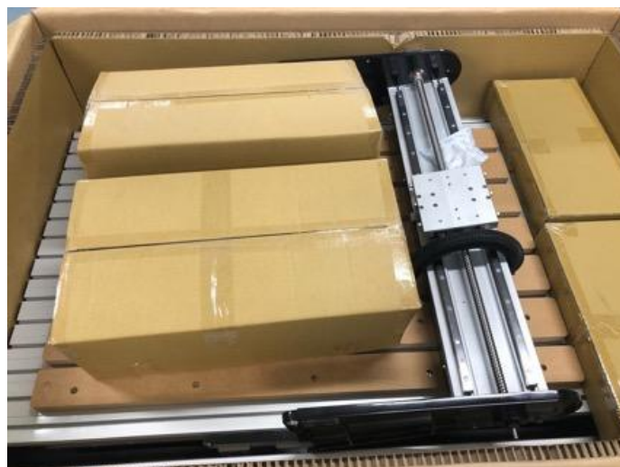
Figure 2: i2R Series-B CNC with box cover removed and ready for lifting
