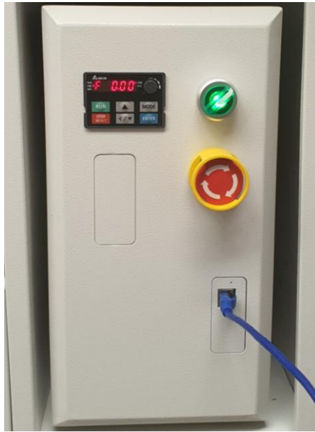
Figure 7: Turn on the power button and plug in Ethernet connector into PC and controller
