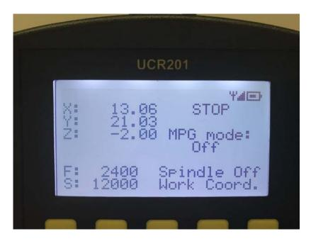
To select an axis to jog press the Axis/FRO/SRO button and then first the X axis getting selected and pressing the same button again toggles through the other axes and finally the FRO and SRO values.
